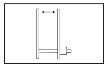
Make the distance between the walls slightly larger than the width of your label
