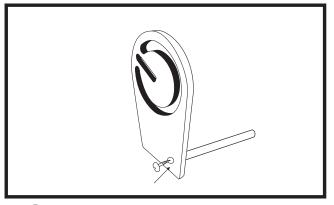
1) Hold the shaft against the hole in the guide wall and screw in place
