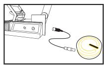
Plug applicator cable in to applicator and Interface.
