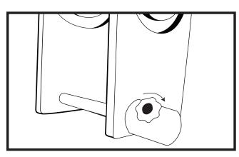
Turn the nob to tighten the screw to hold the shaft in place
